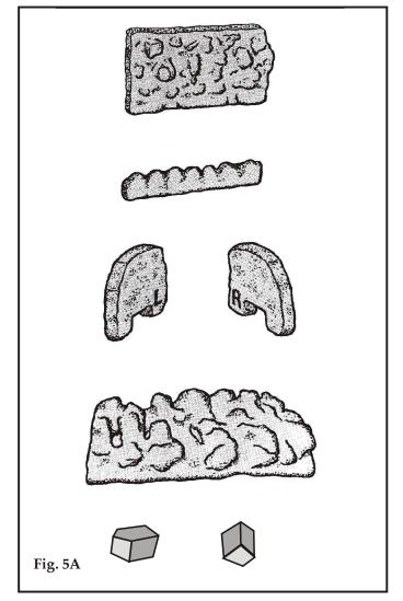
Correct arrangement of the coals is essential to ensure safe operation of the fire. DO NOT INSTALL THE FIRE WITH BROKEN OR MISSING COALS. For replacement of Rear Coal Bed and Centre Coal refer to Section 7 of the Servicing Instructions.
