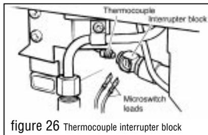
figure 26 Thermocouple interrupter block
