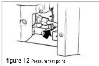
figure 12 Pressure test point
