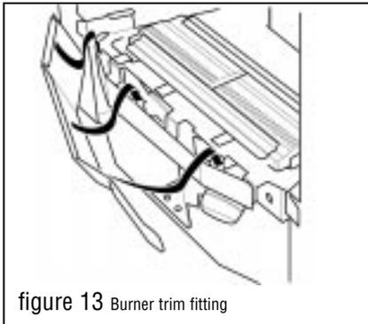
figure 13 Burner trim fitting
