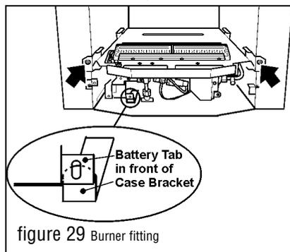
figure 29 Burner fitting
