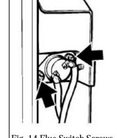
Fig. 14 Flue Switch Screws
