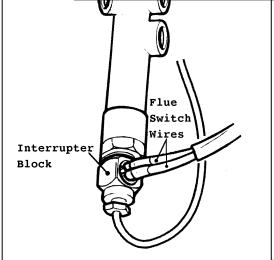
Fig. 13 Flue Switch Wires & Interrupter Block
