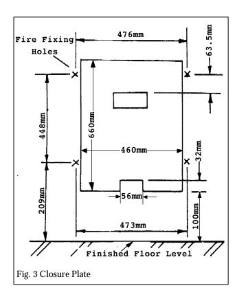
closure plate must be clear and not covered by tape.
