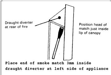
Fig. 9 Spillage Test
