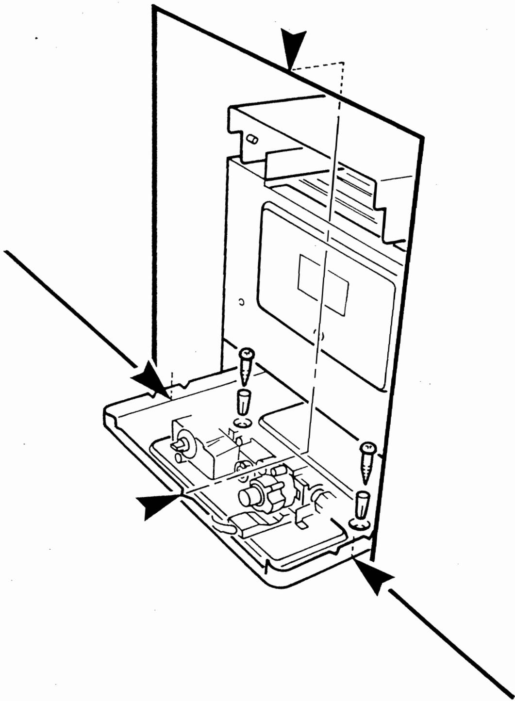
**Back Boiler Fixing Position**
