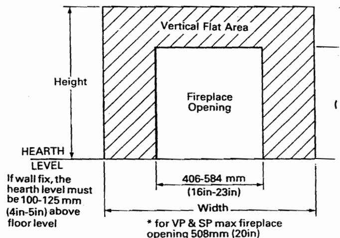
If the opening is being purposely prepared the maximum dimensions are strongly recommended. If the fireplace opening is to the minimum dimension it may be necessary to use the pipe access holes to make the pipe connections.
