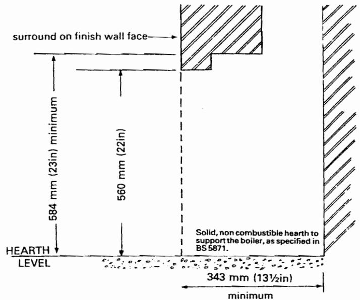
When correctly installed the centre line of the boiler flue socket will be 258 mm-305 mm from the surround on finish wall face.
