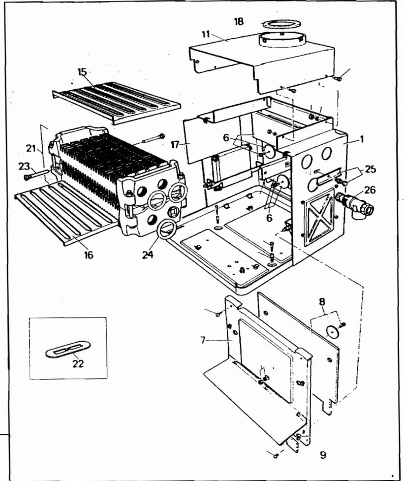
**Boiler and Combustion Chamber**
