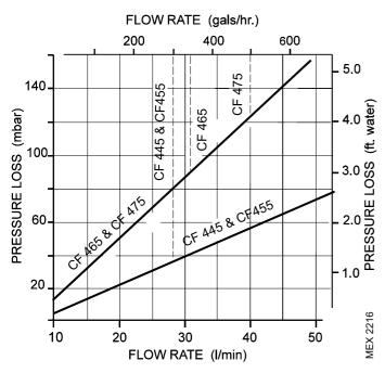
Dotted lines indicate flow rates equivalent to a temperature rise of 11  $^{\circ}C$  (20  $^{\circ}F$ )
