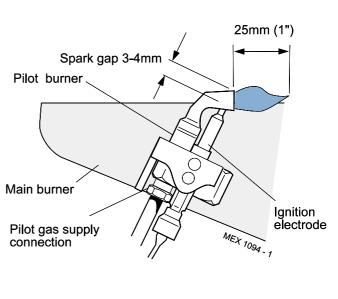
Detail of pilot flame length and spark gap
