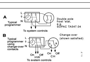
Diagram A shows a double pole frost thermostat, which should suffice for all systems which do not use the OFF terminals of the programmer.
